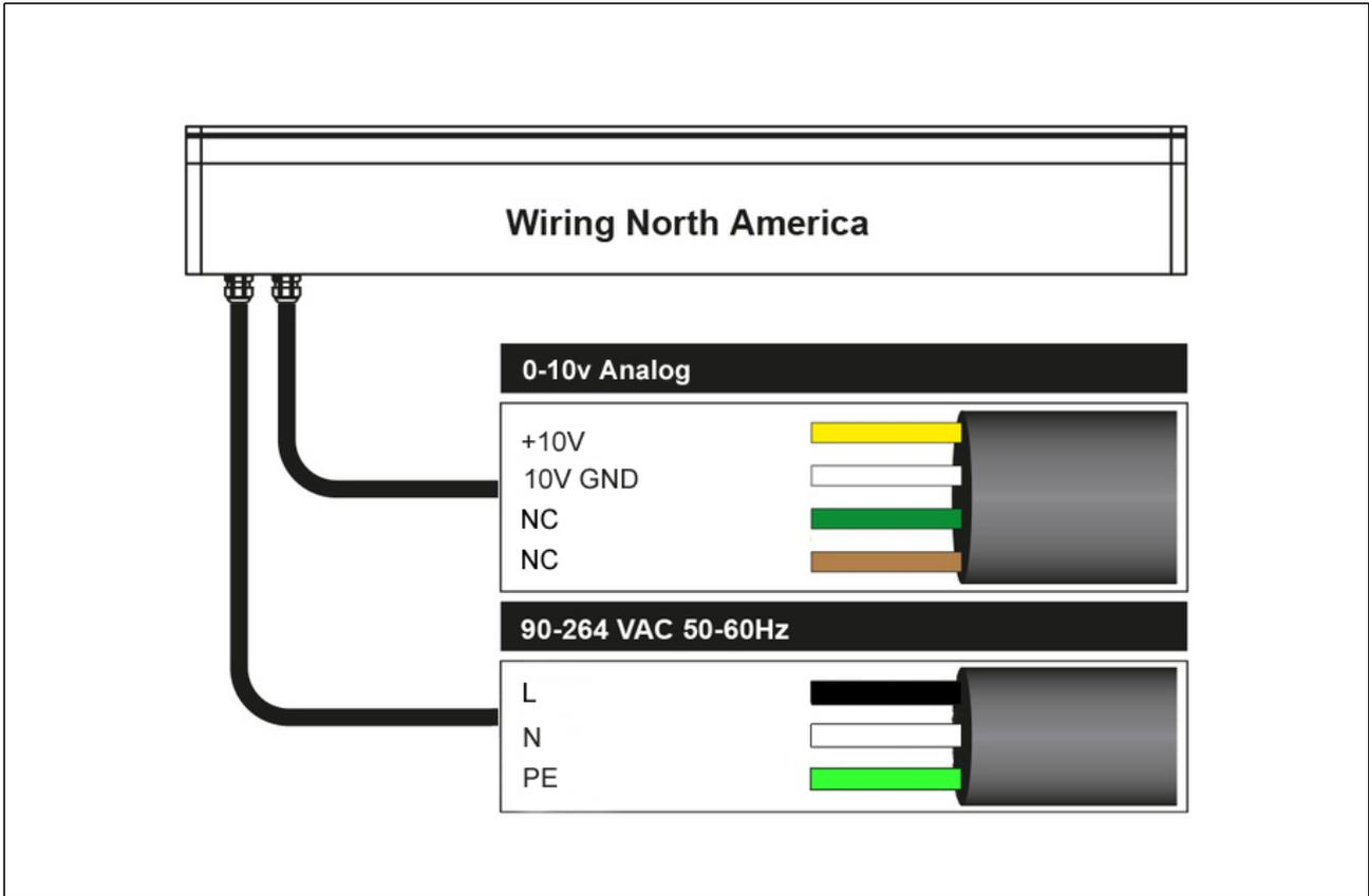
The luminaire connection must be made outside the recess housing by means of a connection sleeve supplied by others. Connect lead mains supply cable with mains supply cable tightly. 0.3 meters of cable must be left in the recess housing for lifting out the luminaire. Strain relief the cable connection. Install the cable only in suitable tubes not directly in the ground. Insert the luminaire housing into the recess housing. Tighten locking screws firmly.
