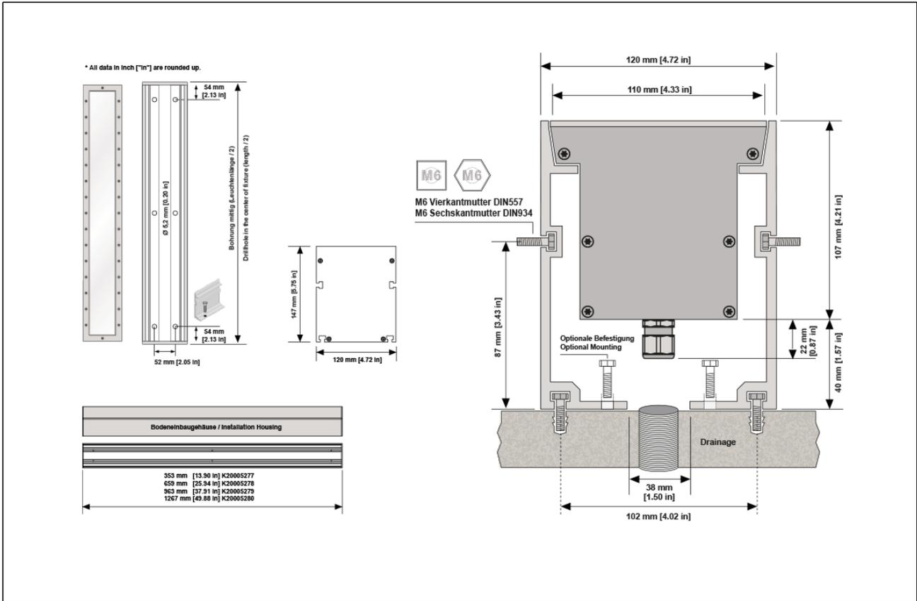
The luminaire must only be operated with the complete protective cover. The support for the housing must be load-bearing for the final use.
